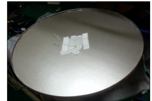
<Before Improvement : Asbestos Tape Finish After Insertion>
